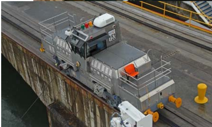
The gear driven locomotives (left) that are used to move the ships through the lock are called “mules”.
